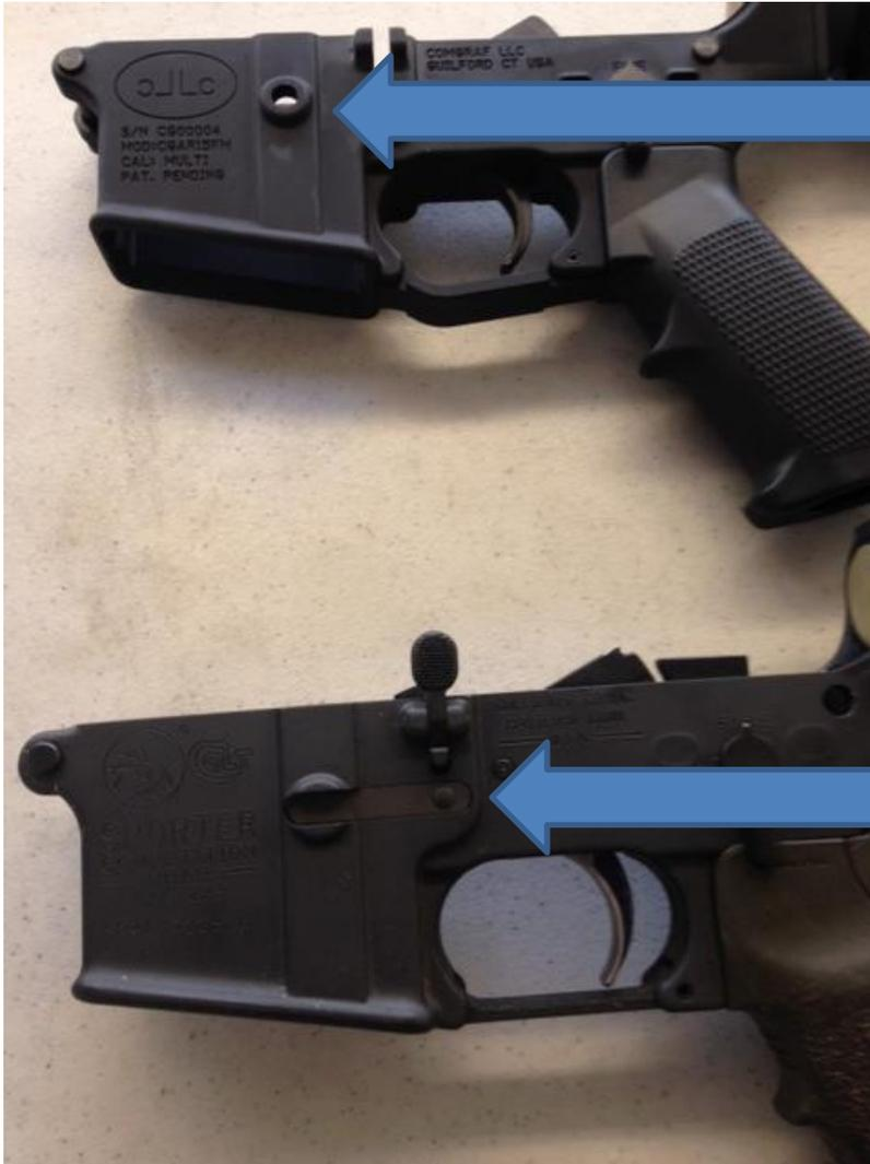
This view shows the left side of the ComGraf fixed magazine lower receiver with no cut-out for the magazine retention bar. It instead has a special hole for a screw which captures a blind nut to fix the magazine in place.
