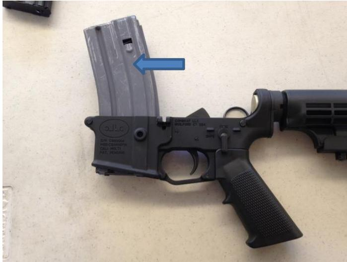
Attempts to insert a curved high capacity magazine into the ComGraf lower receiver were not successful from either the top or the bottom of the receiver as the magazine well geometry has been changed. And, additionally, there is no provision for any of the parts which retain a detachable magazine as the ComGraf lower receiver uses a completely different blind nut assembly to affix the magazine, which nut requires disassembly tools to remove.
