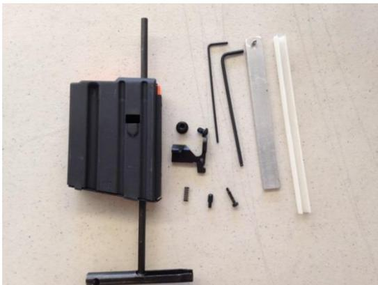
This picture illustrates a 10-round magazine removed from the rifle for cleaning showing the number of special removal tools, including an assembly rod, that were used for removal of the fixed magazine. The process of removing the magazine for cleaning took me around 5 minutes and then it took a few more minutes to re-insert it. The upper portion of the receiver then had to be re-attached. By contrast I can change a magazine in a normal AR15 in a matter of seconds.
